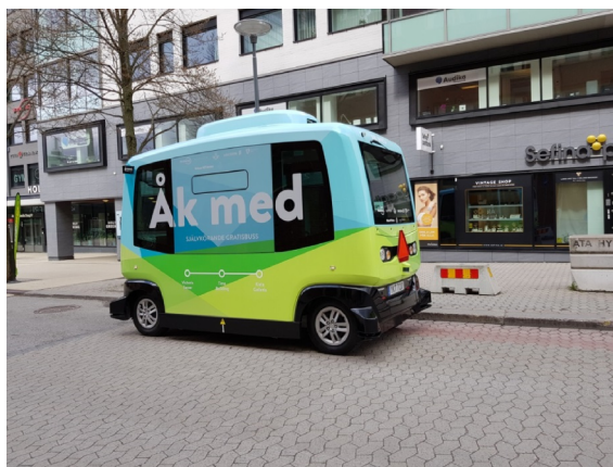
Fig. 3. An EZ10, the small automated bus used in the trial operation in Kista, Stockholm (SARA 1 Research Team, 2018).
